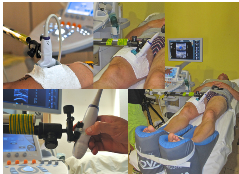
Fig 2. Measurement protocol and subject positioning. An articulated arm ensures that no contact occurs between the transducer and the thigh. Acoustic coupling is ensured using a home-designed silicon pool conforming to the shape of the leg that is filled with bubble-free acoustic gel. All subjects were placed in the supine position using a feet holder to ensure that the quadriceps femoris muscle remained at rest. To maximize inter-day reliability and hasten re-positioning, 4 indelible skin lines were traced during the Pre session (with a waterproof marker). The first line extended across the thigh and was drawn 15 cm above the upper edge of the patella, perpendicular to the patella-ASIS (anterior superior iliac spine) axis. The remaining three lines were drawn parallel to the longitudinal axis of the center of each of the three muscle heads (RF, VM, VL). Per the PLOS ONE policy regarding papers including identifying or potentially identifying information, each subject was informed of the terms of the PLOS open-access (CC-BY) license and provided permission for the publication of these details under the terms of the license.
