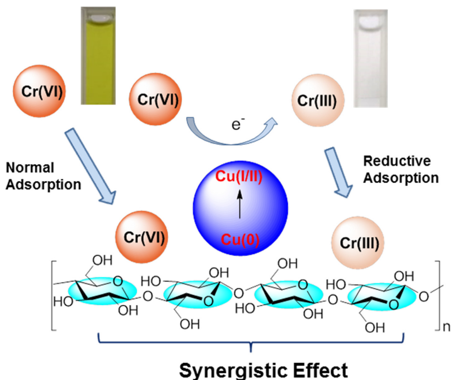
Figure 12. Schematic illustration of Cr(VI) removal by nZVC@PS using synergistic effect (Kumar et al., 2021).
