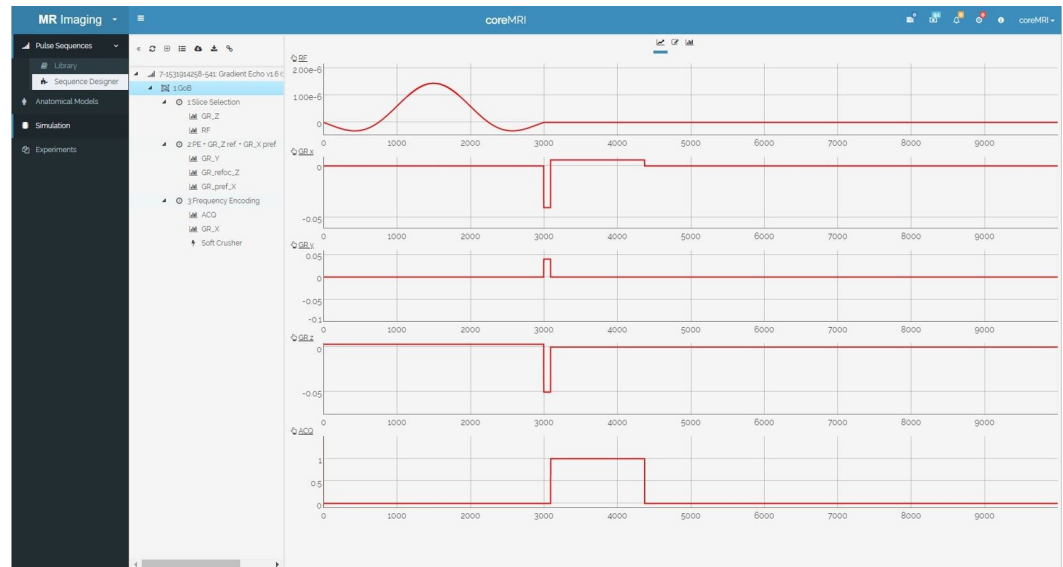
Fig 8. Pulse sequence designer. The web-application of the Pulse Sequence Designer and the graphical representation of the first Group of Blocks (GoB) of the 128x128 Gradient Echo pulse sequence.
