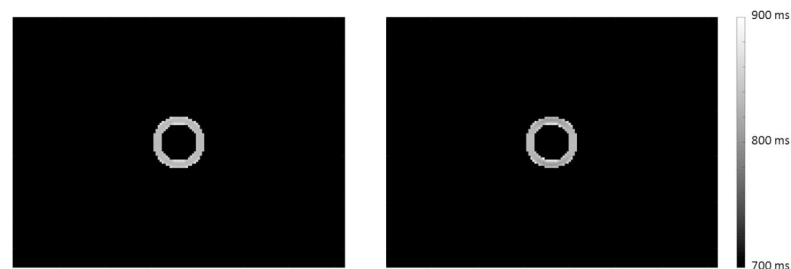
Fig 16. T1 maps of the computer model of the myocardium after the application of the MOLLI pulse sequence. The left image depicts the T1 map without the application of the B0 inhomogeneity map, whereas the right image presents the T1 map with the application of a B0 variation of \pm 150 Hz across the phantom diameter along the PE direction. Note artifactual local variations in the estimated T1 across the phase-encoding direction on the computer model in the right image. The kernel execution time on a p2.xlarge instance was 115 s with and without the application of the B0 inhomogeneity map.
