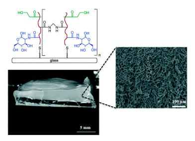
**Figure 7.** Glass-bound glycopolymer based hydrogels used as a model mucin network mimics in recreating the mucosal surface interfacial property. Scanning electron micrographs clearly shows highly porous structure of the hydrogels, these structures mimics membrane-bound mucin networks that were formed from glycoprotein chains. Reprinted with permission from Reference [201]. Copyright © 2015, The Royal Society of Chemistry.
