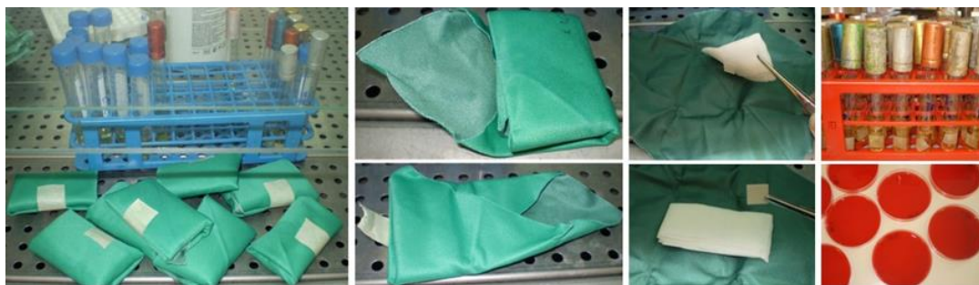
Figure 4. Sterilized packs stored in the warehouse for a period of 1 and 2 months. Presentation of the inside of the pack: gauze and filter paper “Whatman No 1” with a dimension of 1 \text{ cm}^2 which is put into a test tube with brain–heart broth after which it is planted on blood agar.
