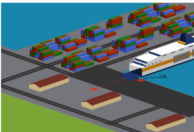
Figure 3. Measurement positions for loading/unloading operations.
