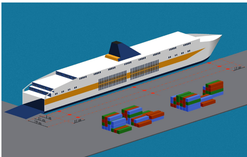
Figure 1. Measurement positions for moored ship in stationary conditions.
