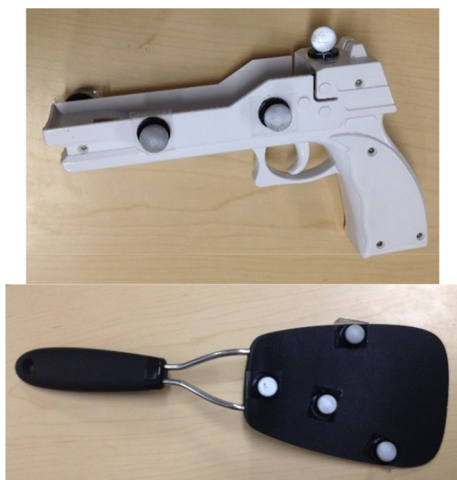
Fig. 2 Objects held during the experiment. The markers were affixed to the objects to track the participants' movements
