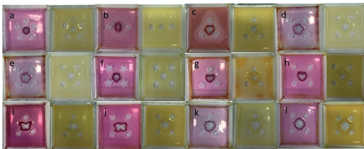
Fig. 7 More complex hydrogel patterns fabricated using the 0.20 mmol HCl (pink) and GdL (yellow) hybrid gels with DBS-carboxylate loaded into the central reservoir. Gel objects (not pictured) could be obtained by cutting and removing the structures from the surrounding gel. (a) Circle surrounded by 5 circles, (b) circle surrounded by 2 circles, (c) star surrounded by 3 circles, (d) star surrounded by 4 circles, (e) star surrounded by 4 circles, (f) star surrounded by 4 stars, (g) moon surrounded by 3 circles, (h) moon surrounded by 4 circles, (i) butterfly surrounded by 3 circles, (j) butterfly surrounded by 4 circles, (k) flower surrounded by 3 circles, (l) flower surrounded by 4 circles.
