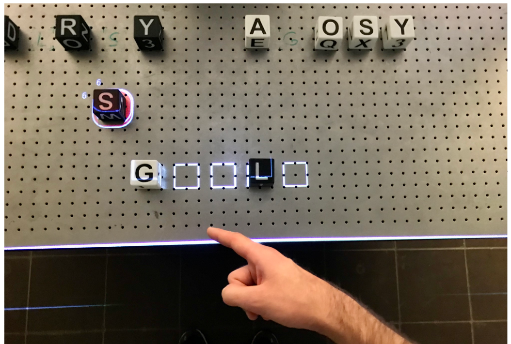
Figure 14. Pointing gesture: User points to cube [S], which is enveloped by the laser pointer.
