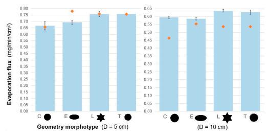
**Figure 4.** Mean evaporation flux for filter paper models with leaf-inspired morphotypes, for two characteristic dimensions (control circle D = 5 and 10 cm). Error bars represent ±1 SD. Orange markers represent theoretical estimates based on L<sub>eff</sub> (Equation (2)), for t<sub>model</sub> = 28 °C and v<sub>air</sub> = 0.015 m/s.
