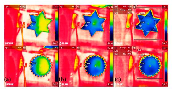
**Figure 5.** Thermal time-lapse of evaporating models of lobed and toothed shapes (characteristic dimension 10 cm): (a) Shortly after cap removal (evaporation release); (b) 1 min after; and (c) 20 min after.
