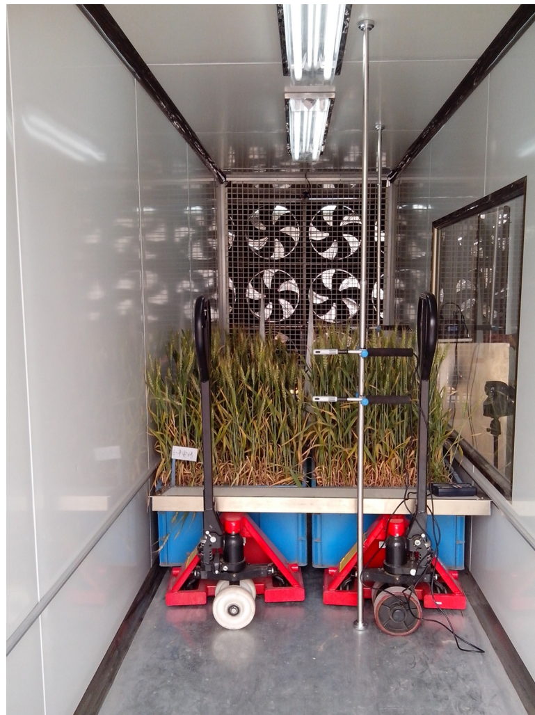
Fig 3. Wind tunnel simulation of lodging resistance in wheat.
