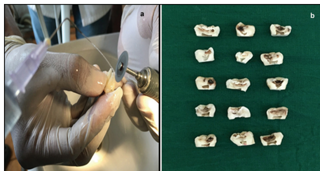
Figure 1: a. sectioning of the tooth samples using a diamond disc; b. sectioned samples
