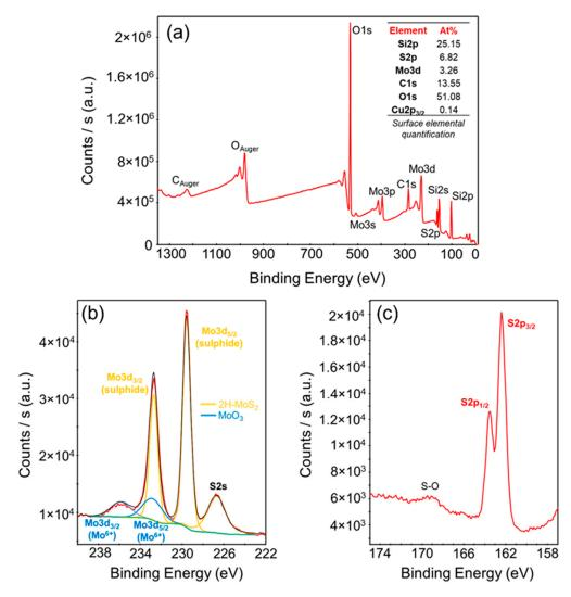
**Figure 3.** (a) Survey XPS spectrum of  $MoS_2$  on  $SiO_2$  produced by sulfurization of the 2.8 nm  $MoO_3$  film, with the indication of the evaluated surface elemental composition. (b) XPS spectra of the Mo 3d and S 2s core levels, with the deconvolution of the  $Mo^{4+}$  contribution (related to  $MoS_2$ ) and the  $Mo^{6+}$  contribution (related to residual  $MoO_3$ ). (c) S 2p core levels spectra, indicating the predominance of the sulphide contribution, with a small S-O component.
