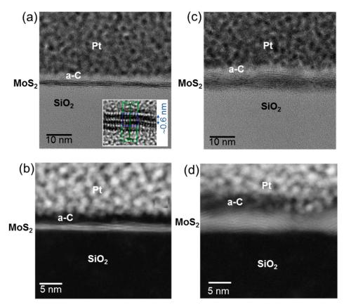
**Figure 4.** Cross sectional HR-TEM (a) and HAADF-STEM (b) images of few-layers  $MoS_2$  obtained by sulfurization of the ~2.8 nm  $MoO_3$  film on the  $SiO_2$  substrate.  $MoS_2$  is composed by nearly horizontally aligned 2–3 layers. The interlayer spacing in a 3-layers region is evaluated from the HR-TEM in the insert of panel (a). Cross sectional HR-TEM (c) and HAADF-STEM (d) of multilayers  $MoS_2$  obtained by sulfurization of the ~4.2 nm  $MoO_3$  film.
