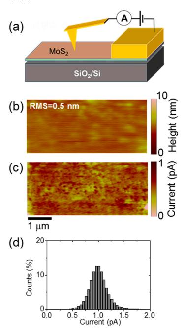
**Figure 7.** (a) Schematic of the C-AFM setup for local conductivity mapping of few-layers  $MoS_2$  on  $SiO_2$ . (b) Morphology and (c) current map simultaneously measured with tip-to-sample bias of 5 V. (d) Histogram of current values from the C-AFM map.
