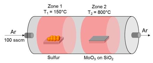
**Figure 1.** Schematic illustration of the sulfurization process of the thin  $MoO_3$  films on the  $SiO_2/Si$  substrates.
