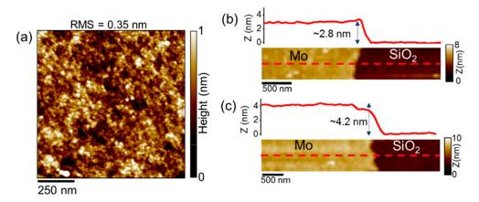
**Figure 2.** (a) Typical AFM morphology of as-deposited MoO<sub>3</sub> thin films on SiO<sub>2</sub>, with the indication of the root mean square (RMS) roughness. (b,c) Determination of the thickness of films deposited with two different sputtering times by measurement of the step heights ( $\sim$ 2.8 nm and  $\sim$ 4.2 nm) with respect to SiO<sub>2</sub> on scratched regions.
