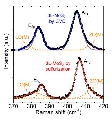
**Figure 8.** Raman spectrum for 3L-MoS<sub>2</sub> produced by sulfurization (red), compared with a reference spectrum for CVD grown 3L-MoS<sub>2</sub> (blue). Data for CVD 3L-MoS<sub>2</sub> were adapted with permission from [65], copyright Elsevier 2020.
