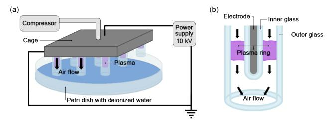
**Figure 7.** (**a**) Scheme of the dielectric barrier discharge (DBD) device and of the experimental set-up. (**b**) Details of one of the 13 electrode–glass tube components.
