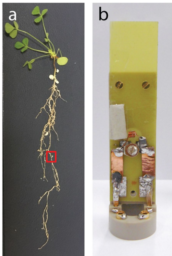
Figure 1. Photograph of M. truncatula root system and custom-designed home-built microcoil. (a) Photograph of a representative M. truncatula plant (five weeks old, three weeks post inoculation). Typical root nodule indicated with a red square. Some white perlite beads are still visible along the root system. (b) Photograph of a home-built solenoid coil insert mounted on a Bruker insert holder. The solenoid inner diameter is 1.5 mm; further details are described in the materials and methods.
