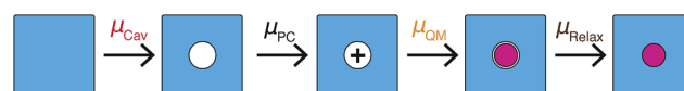
Fig. 2 Schematic of the partitioning of the single ion solvation free energies used here. The contributions are the cavity formation, point charge, quantum mechanical and hard sphere relaxation terms.
