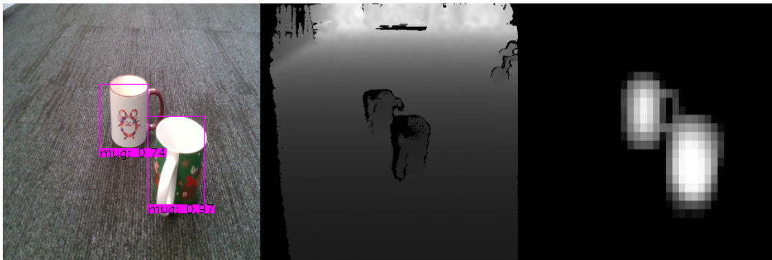
Figure 13. An example of real world object classification using the proposed network model: segmented and classified RGB frame (left), depth frame (middle), and predicted depth mask (right).
