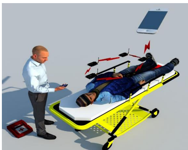
Figure 2. Wireless body sensor network communicating through a mobile phone.
