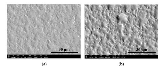
**Figure 1.** Scanning electron microscopy (SEM) images of nanoparticles distribution: (**a**) silver nanoparticles and (**b**)reduced graphene oxide flakes in chitosan/chondroitin sulfate (Chi/CS) film.
