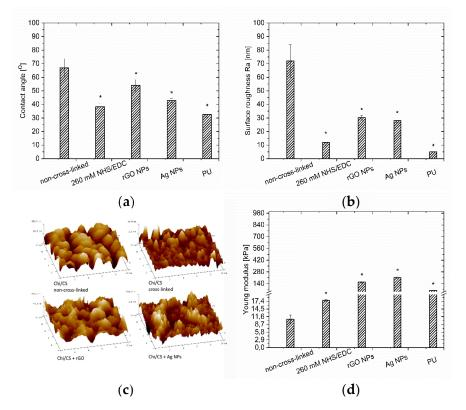
**Figure 2.** Properties of the Chi/CS films and polyurethane (PU) control: (**a**) wettability; (**b**) surface roughness; (**c**) thickness; (**d**) stiffness. Results obtained for non-cross-linked, 260 mM NHS/EDC (N-hydroxysulphosuccinimide/1-ethyl-3-(3-dimethylaminopropyl) carbodiimide) cross-linked films and samples modified with nanoparticles. The data represent mean  $\pm$  SD, n = 8; \* p < 0.05 vs. non-cross-linked sample.
