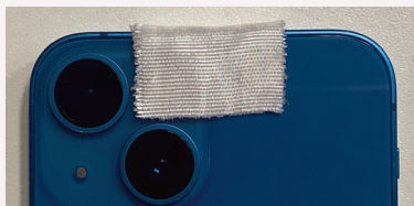
Figure 6 Six layers of micropore tape were applied to reduce the intensity of the flash of this phone
