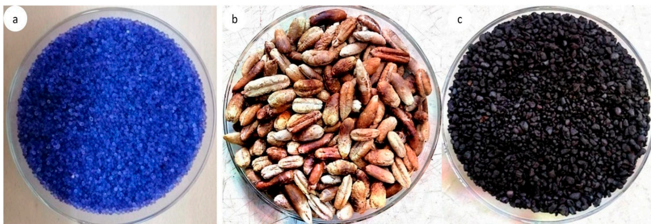
Figure 2. (a) Silica gel type III, (b) dried date stone and (c) activated carbon (AC).
