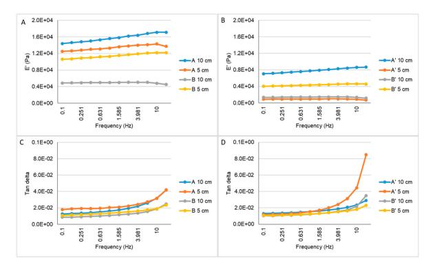
**Figure 2.** Storage modulus (**A** and **B**) and tan delta (**C** and **D**) under dynamic compression solicitation versus the increasing frequency, ranging from 0.1 to 10 Hz for Coll/nanoHA scaffolds produced with different collagens before (A and B) and after sterilization (A' and B').
