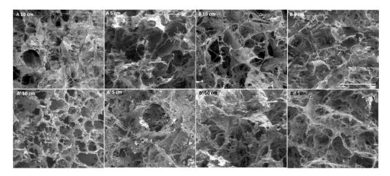
Figure 1. SEM images of Coll/nanoHA scaffolds A–B and A'–B'. Scale bar: 500 µm.
