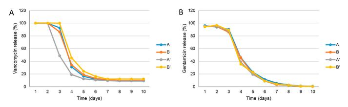
**Figure 5.** Vancomycin (**A**) and gentamicin (**B**) concentrations present in the solution released from Coll/nanoHA samples with and without sterilization, at different time points until 10 days.
