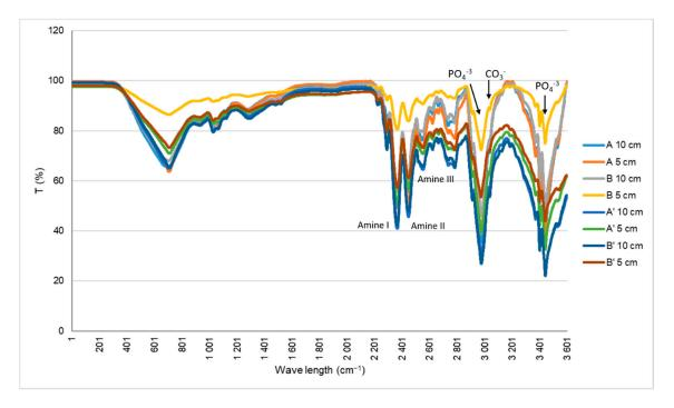
**Figure 3.** FT-IR spectra of the Coll/nanoHA scaffolds produced with different collagens before (A and B) and after sterilization (A' and B').
