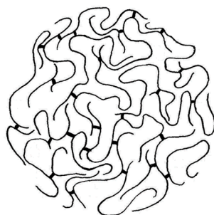
Figure 1. Adaptation of the macromolecular “microgel” structure proposed in 1960 [8] to describe a ligninsulfonate crosslinked polymer chain (sulfonate groups omitted).
