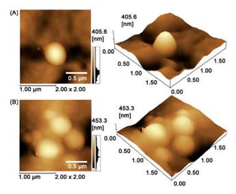
**Figure 1.** Atomic force microscope (AFM) 2D and 3D images. **(A)** Free drug nanoparticles and **(B)** MET-loaded PLGA (metformin-loaded poly lactic-*co*-glycolic acid) nanoparticles. The topography was observed in water with a frequency shift of 1 Hz and a cantilever oscillation amplitude of 2  $\mu$ m  $\times$  2  $\mu$ m. The scale indicates the topographic height.
