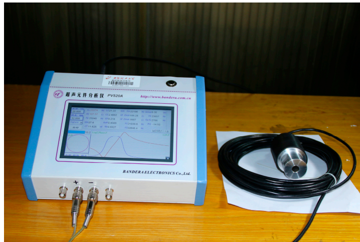
Figure 10. The impedance test of the sandwiched ultrasonic transducer.
