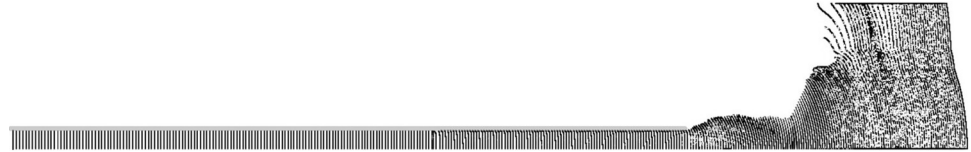
Fig 8. The planarity of the shock front is largely lost at the shock tube exit. The edge of the shock front at each time step ( \Delta t = 38.5 \mu s ) from t = 0-13.5 ms in the moderate strength shock in a mid-wall cut. As the shock exits the shock tube, denoted by a grey bar, the shock front loses its planar nature and expands, becoming non-planar.
