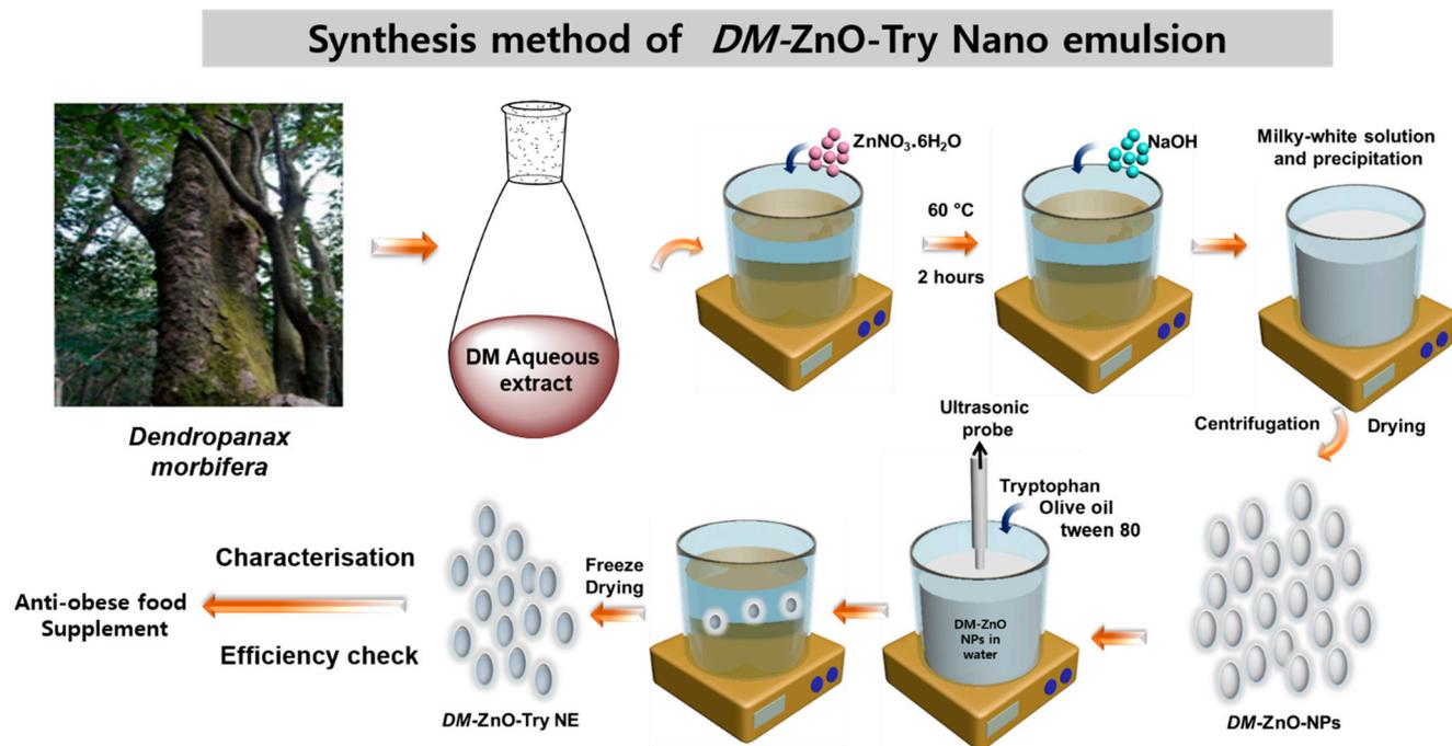
Figure 1. Preparation of DM-ZnO-tryptophan, oil in water nanoemulsion using the ultrasonication method.
