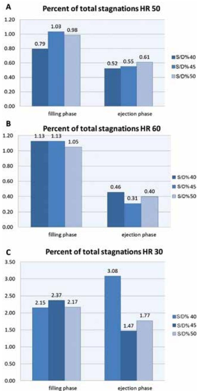
**Fig. 5 - PED45**, percent of total stagnations for the following parameters: S/D% 40, S/D% 45 and S/D% 50 and (A) HR 50, (B) HR 60, (C) HR 30.
