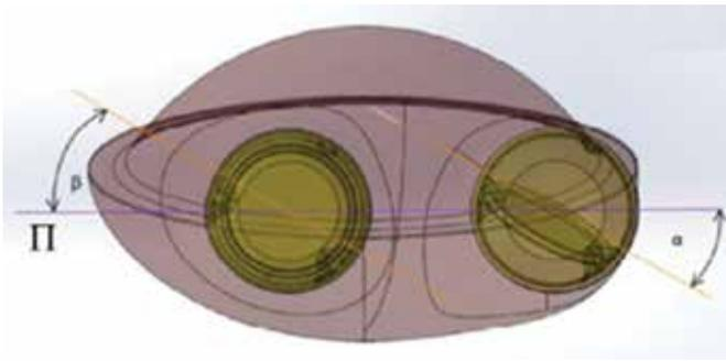
Fig. 3 - Definition of the angular position of valves (18).
