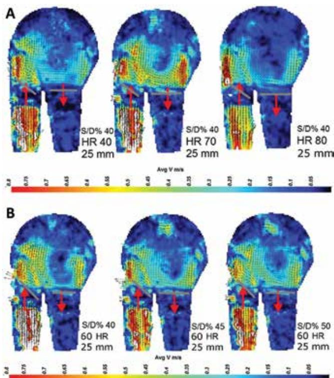
**Fig. 6 - PED30:** (A) a flow comparison for different heart rates at S/D% 40; (B) a flow comparison for different systole to diastole percentages at HR 60.
