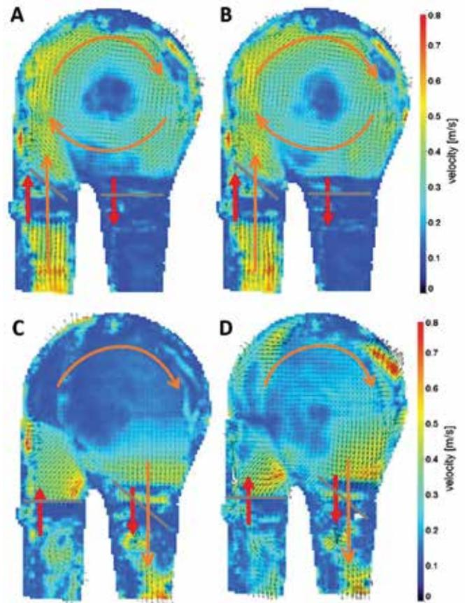
Fig. 4 - PED45, velocity distribution: (A) filling phase, HR 40, S/D% 45; (B) filling phase, HR 40, S/D% 50; (C) ejection phase, HR 30, S/D% 40; (D) ejection phase, HR 60, S/D% 40.
