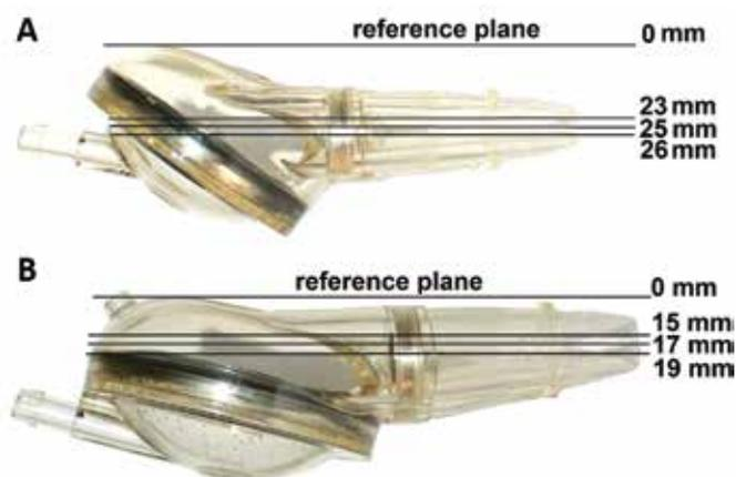
Fig. 1 - Measurement planes: (A) PED 30, (B) PED 45.
