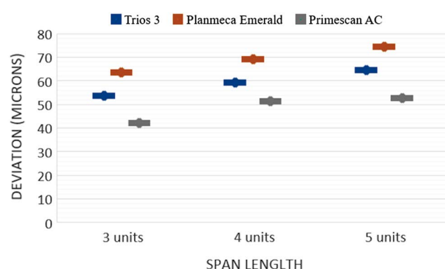
Fig. 5. Precision of intraoral scanners in relation to different span lengths.
