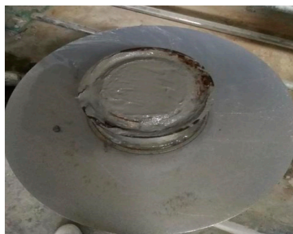
Figure 3. Slump test of P1.
