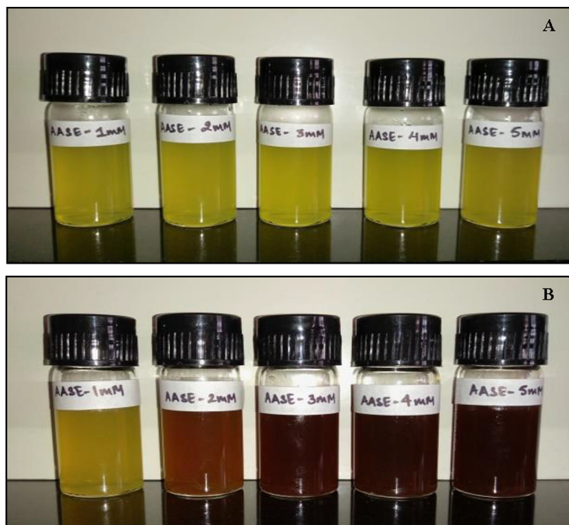
Fig. 2. Colour change in Achyranthes aspera stems extract (AASE)-Silver nitrate mixtures at different concentration (1–5 mM) indicating synthesis of silver nano-composites; (A) Initial mixtures; (B) Final mixtures.
