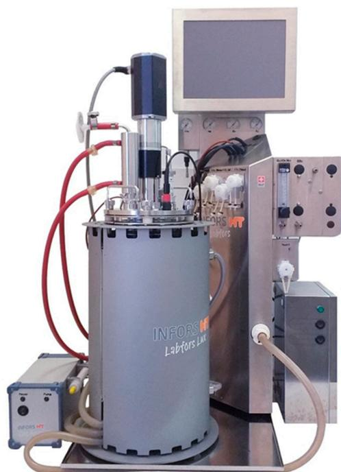
**Figure 6.** The Labfors 4 Lux photobioreactor (Infors HT, Switzerland) used in this study.
