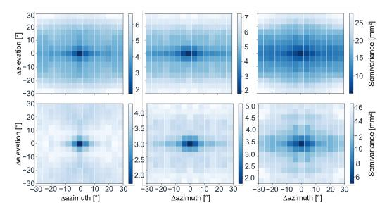
**Figure 3.** The 2D variogram maps of the residuals for the antennas TRM5 (**left**), AV 28 circular ground plane (**middle**), and AV28 rectangular adaptor (**right**), before (**top**) and after (**bottom**) removing the elevation pattern.
