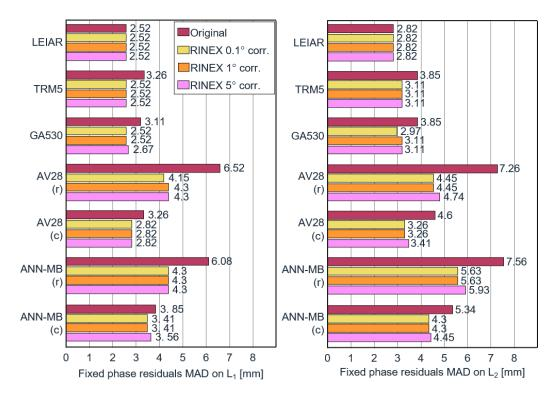
**Figure 2.** Ambiguity-fixed phase residuals on  $L_1$  (**left**) and  $L_2$  (**right**) before and after the calibration using  $0.1^{\circ}$ ,  $1^{\circ}$ , and  $5^{\circ}$  binning widths. The abbreviations (c) and (r) in the antenna names correspond to the utilized mounting brackets (circular plane and rectangular bracket).
