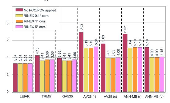
L<sub>1</sub>L<sub>2</sub> Up-MAD (after subtracting different antenna bracket heights) [mm]
