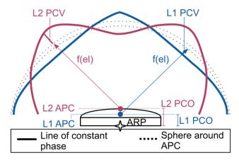
**Figure 1.** Schematic illustration of Antenna Reference Point (ARP, black star symbol), Antenna Phase Center (APC, filled circles), lines of constant phase (solid colored lines), and spheres around APC points (dashed lines) on  $L_1$  (blue) and  $L_2$  (red). The Phase Center Variations (PCVs, thick colored lines between the spheres around APC and line of constant phase) are shown as functions of the elevation f(el) on the respective frequency.
