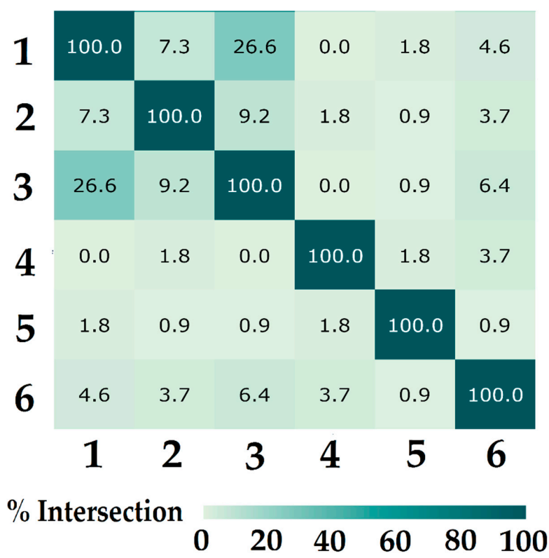
Figure 5. Comparison matrix of the examined samples. The values in each cell represent the percentage of statistically significant overlap for the confidence intervals across all analyzed peaks for each pair of samples.
