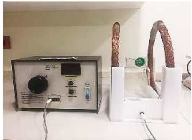
Figure 1. The magnetic field generator (Amen Ara @ Ni200A) composed of Helmholtz coils and current controller system. The Helmholtz coils consists of two identical coils with diameter of 22 cm with 22 cm axial separation distance. By altering the current delivered to coils, the magnetic field generated by coils was adjusted to desired value (1 mT). The magnetic field intensity was calibrated at 1 mT by a field strength meter
