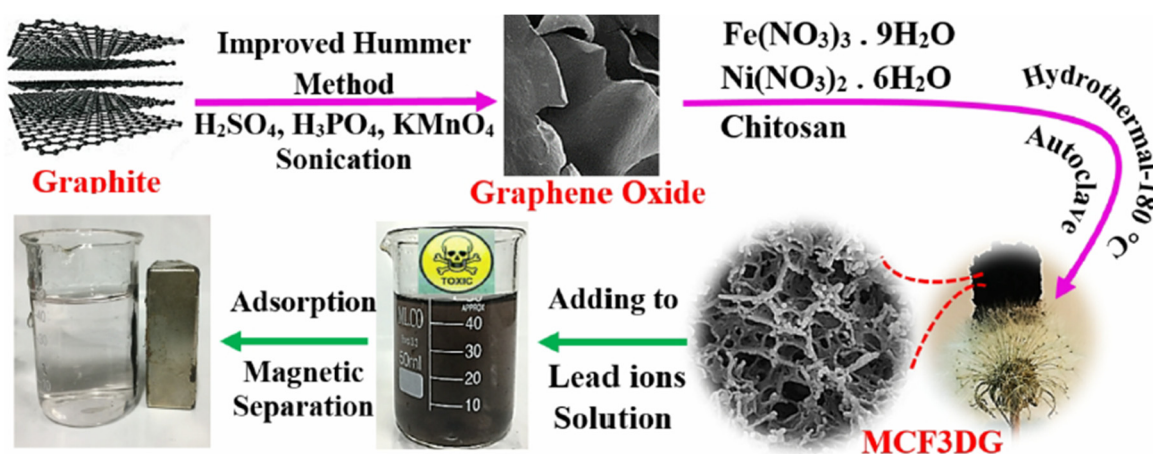
Figure 9. Synthesis of magnetic chitosan-functionalized 3D graphene nanocomposite MCF3DG (Reproduced or adapted from ref. [62], with permission from American Chemical Society, 2020).
