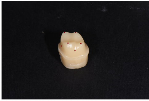
FIGURE 3 Measurement points in triple scanning method; tip of four occlusal surface cusps and midpoints of axial walls
