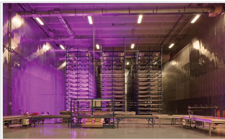
Figure 6. Plant germination room that is a part of the upstream portion of the facility at iBio CMO (formerly Caliber Biotherapeutics).
