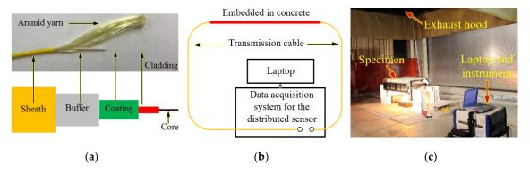
**Figure 2.** Distributed fiber optic sensor: (a) sensor structure, (b) schematic of measurement setup, and (c) photo of setup. A length of the fiber optic cable was embedded in the concrete slab of the specimen.
