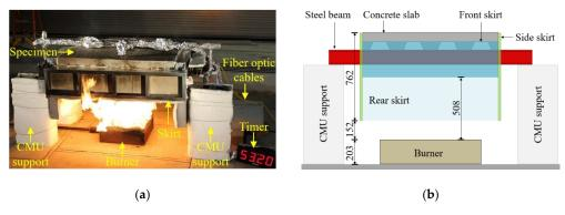
Figure 4. Test setup: (a) photograph, and (b) illustration (units in mm).
