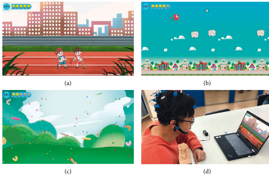
FIGURE 5: Three serious games were developed to improve attention. (a) Tug of War was designed in terms of the mechanism of sustained attention. (b) Adventures of Birds was designed in terms of the mechanism of selective attention. (c) Greedy Jelly was designed in terms of the mechanism of focus attention. (d) A subject playing a serious game with closed-loop neurofeedback.
