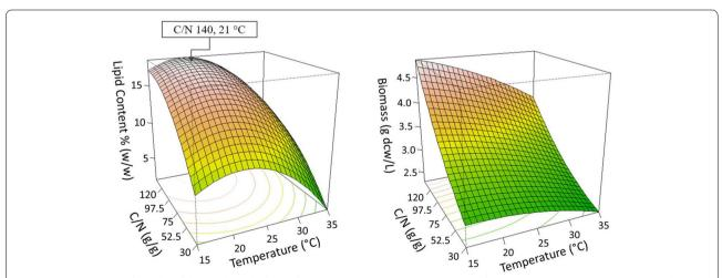
**Fig. 2.** 3D Response surface plot of the combined effects of C/N ratio and temperature levels on (left) lipid content (g lipid weight/g yeast dry cell weight), and (right) growth (g yeast dry cell weight /L) of *Y. lipolytica*. Determined optima are highlighted in the respective plots
