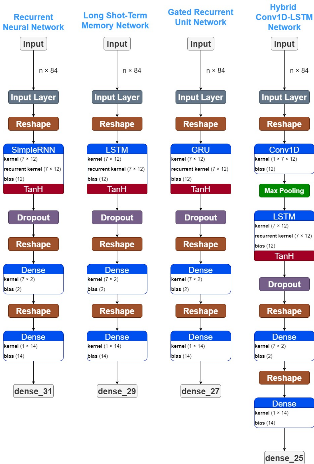
Figure 4. Deep learning architectures for COVID-19 predictions. The notation n is used for the n -th input that is ingested into the model.
