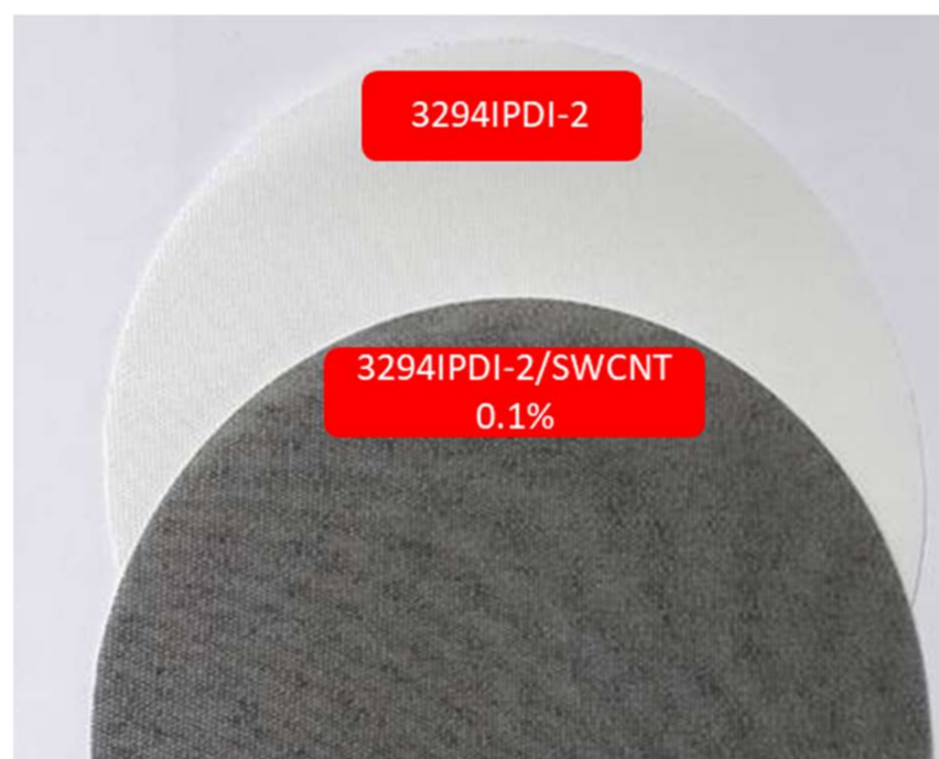
Figure 20. Appearance of UPRON fabric coated with: (top) 3294IPDI-2 and (bottom) 3294IPDI-2 doped with 0.1 wt. % SWCNT.
