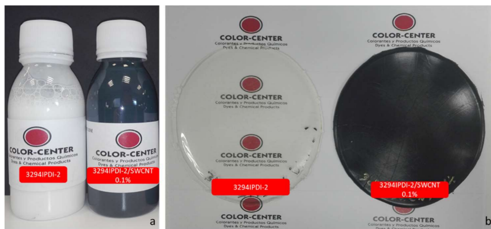
Figure 19. (a): 3294IPDI-2 WPUD dispersion before and after Tuball additivition. (b): casted films obtained after drying and curing in Teflon mold.
