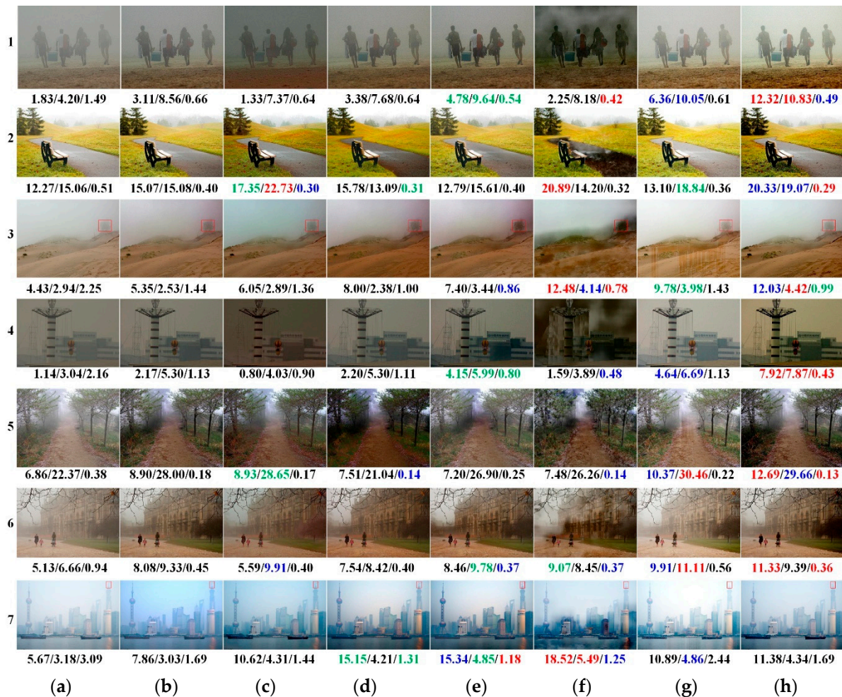
Figure 6. Qualitative comparisons on the LIVE foggy outdoor dataset [33] with average gradient (AG), image entropy (IE), and the fog-aware density evaluator (FADE) values listed below each image. The 1st, 2nd, and 3rd winners of each measurement are displayed in red, blue, and green colors, respectively. (a) Hazy Inputs; (b) DehazeNet [6]; (c) AOD [8]; (d) colour attenuation priors (CAP) [2]; (e) proximal dehazing network (PDN) [10]; (f) grid dehazing network (GDN) [11]; (g) F-DCP [15]; (h) TGL-Net-Mix.
