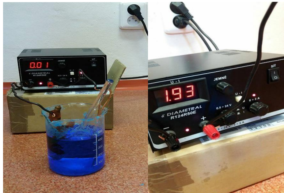
Figure 1. Electroplating process on conductive fabric.
