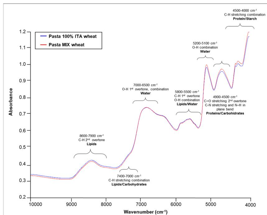
**Figure 1.** Overlay of average FT-NIR raw spectra of pasta classes, i.e., pasta made with 100% Italian wheat (blue trace) and pasta made with a mixture of wheat cultivated abroad (red trace), with fundamental spectral bands.
