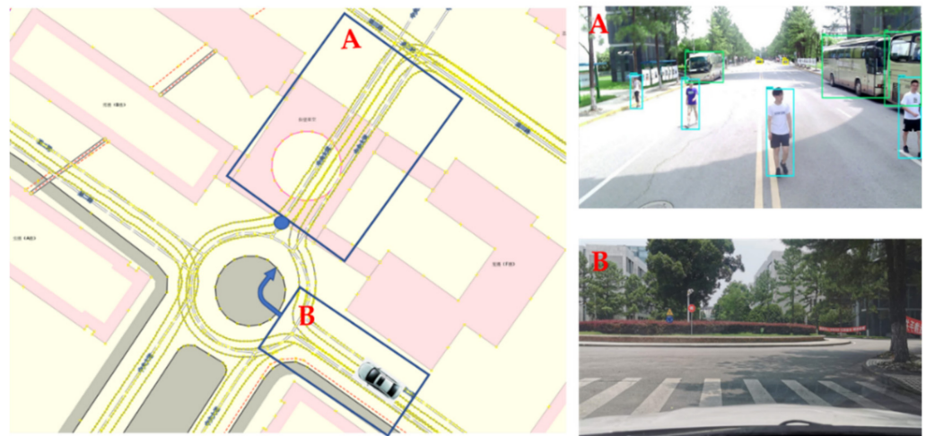
Figure 18. Test scenario for the vehicle-to-infrastructure (V2I) system. The left side is a HD map in vector format from OpenStreetMap. The blue marker is the placement of the roadside unit (RSU).
