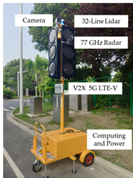
Figure 5. The movable intelligent roadside sensing and computing platform. The sensor unit consists of a radar, a camera, and a 32-line lidar; the vehicle-to-everything (V2X) unit uses the 5G LTE-V communication format; and the computing unit is an Nvidia Xavier.
