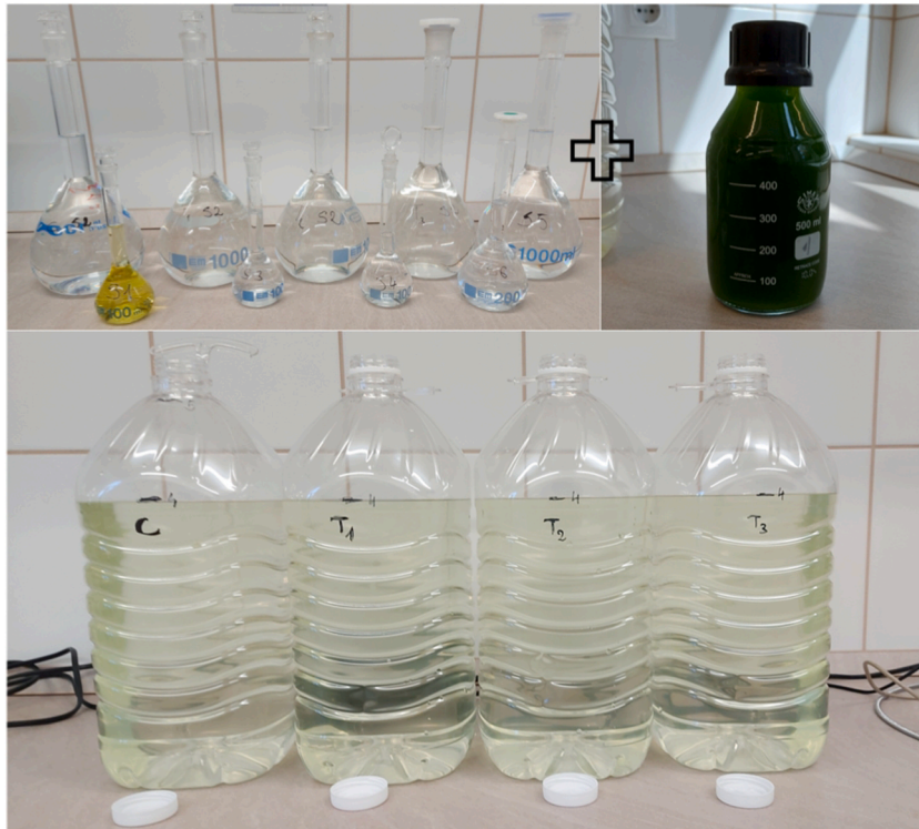
Fig. 2. The prepared stock solutions, the C. vulgaris and the start of the experiment.
