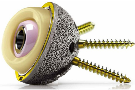
Fig. 1. (A) The G7 dual mobility acetabular system (ZimmerBiomet, Inc, Warsaw, IN) device includes a vitamin-E infused highly crosslinked polyethylene outer head and Delta ceramic inner femoral head. The titanium alloy acetabular cup is a 3D porous cup with a mean pore size of 475 microns, 70% porosity, and a coefficient of friction of 1.25. A multi-hole design for the acetabular cup was used in this case.
