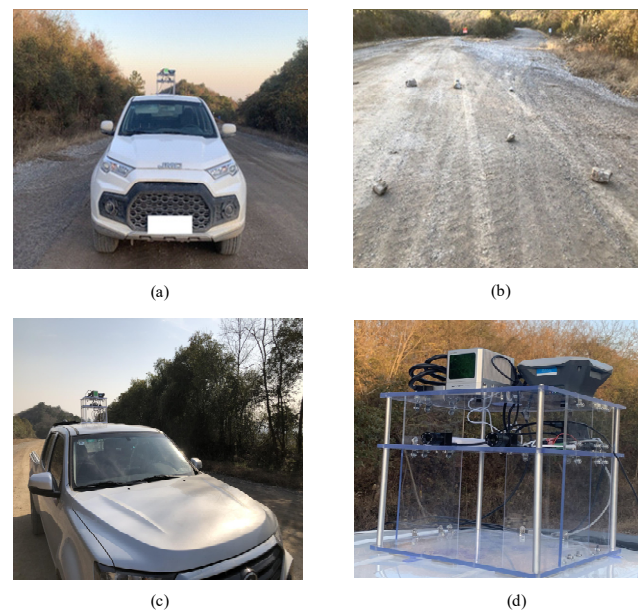
Figure 7. The place where the data was collected in the experiment. (a) Vehicles used in the experiment; (b) randomly placed rocks on the road; (c) side of the vehicle; (d) the detail of the equipment.
